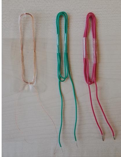
**Figure 3.8:** Antennas used with a frequency of 13.56 MHz other than the RyscCorp antenna.
