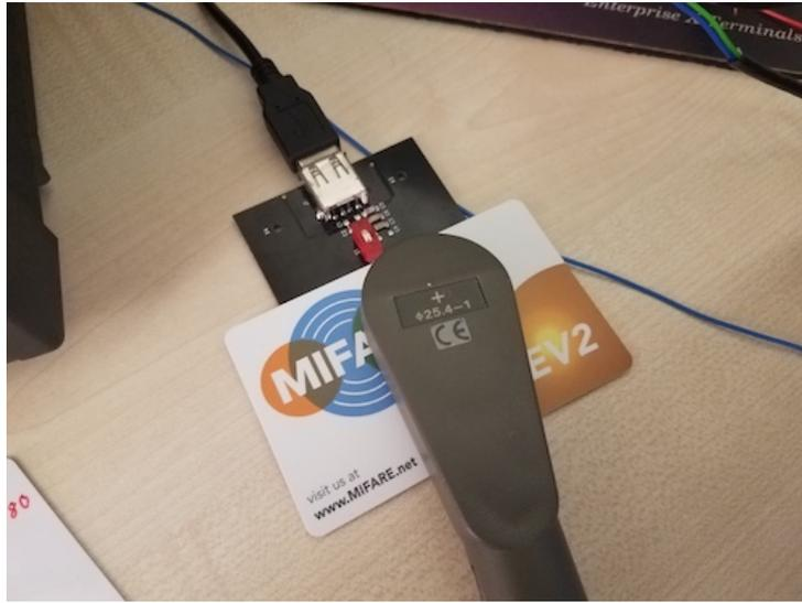
**Figure 3.7:** Eavesdropping a Mifare DESFire REQA transaction using a near-field probe hooked up to a spectrum analyzer.
